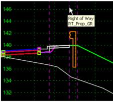
Note that catch slopes for up to 35 MPH design (no guardrail warrant) and over 35 MPH design (with guardrail warrant) are both in our standard library.
